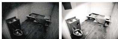
IR LED Illumination in a completely dark room. IR source output: 50mW, wavelength: 850nm @ 5m. IR-Extend models only.
